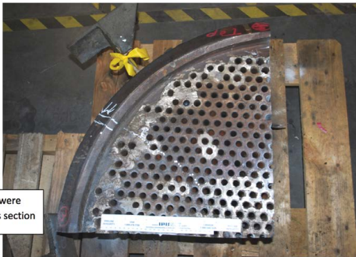
Figure 23. Top channel quarter section, top view
